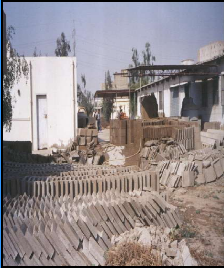
Stock of Precast lining units at CWHR
